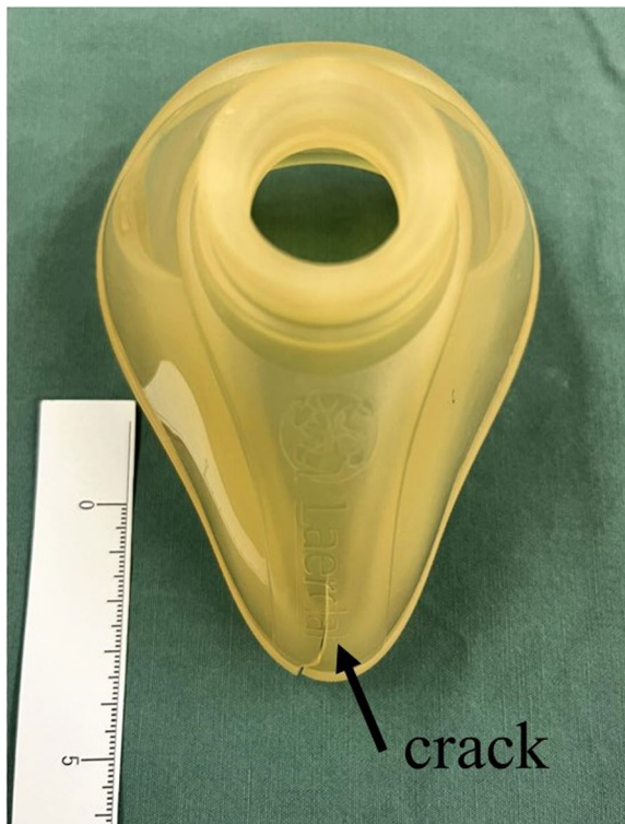
Fig. 1 Anesthesia mask with crack
